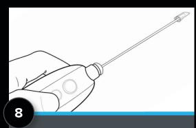
Perform calibration using either button on the handpiece when prompted. Ensure cap is installed.
