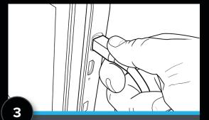
Connect to power adapter or ensure battery level is sufficient for expected procedure duration.
