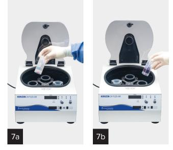
Open centrifuge lid. Place ACP Max counterweight opposite of the ACP Max device. Ensure counterweight matches the weight of blood to be processed. Set the centrifuge rpm to 3000 and time according to volume. 30 mL = 3 minutes / 60 mL = 6 minutes / 90 mL =9 minutes.
