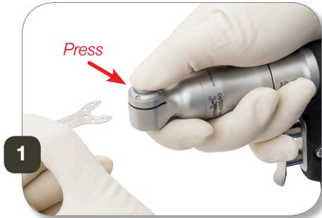
Press the button located on the top of the attachment.
