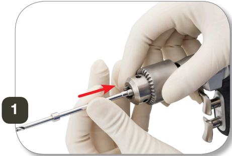
Insert the drill bit into the open drilling chuck.
