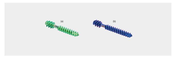
Not just an ordinary headless screw, the RetroFusion implant is designed for arthrodesis and provides compression and strength across the joint. The implant's proximal and distal threads are arranged in opposite directions to pull the joint together when the implant is inserted.
